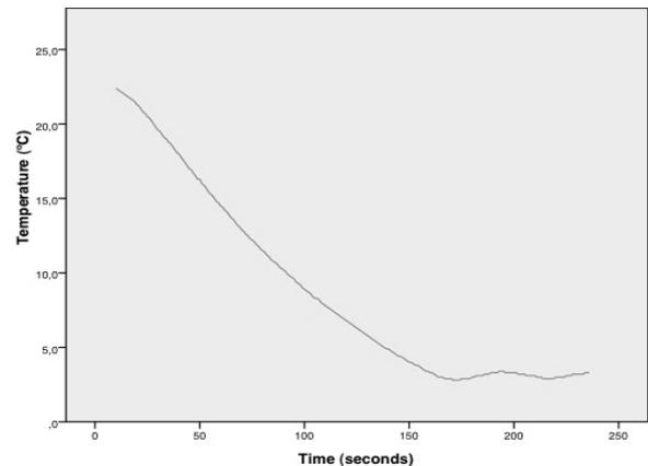
**Figure 2.** Peltier device-epidermis interface temperature during the first 4 minutes.
